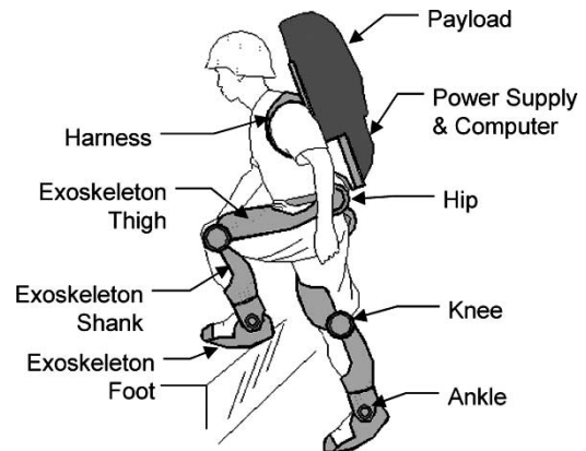
Fig. 1. Conceptual sketch of a lower extremity exoskeleton. Proper actuation of the robotic legs removes the payload weight from the wearer, while allowing the wearer to effortlessly control and balance the machine.
